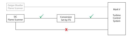
The SiC flame scanner can be fixed on the turbine with the existing mounting options without changing the hardware or making other alterations. Conventional fuels can further be used without any restrictions.
