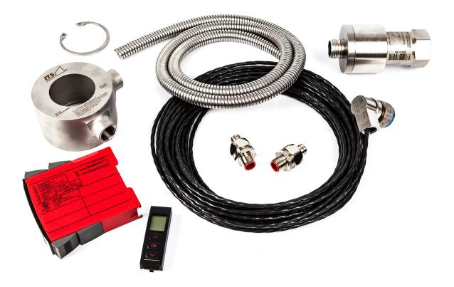
This set protects the flame scanner cable and enables the conversion from the Geiger Mueller principle scanning technology (used in GE261A1812P003 -> GE261A1812P015 etc. or in the Honeywell LG1093AA04 -> LG1093AA46 etc. flame scanners) to the modern SIC flame scanning technology that is used in the ITS 184X0254M029 flame scanner. It also reduces the thermal load with a water cooling system.
